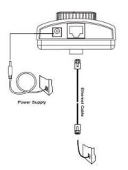
Please verify that your product package contains all the accessories listed in the foregoing Package Contents. Depending on the user's application, an Ethernet cable may be needed. The Ethernet cable should meet the specs of UTP Category 5 and not exceed 100 meters in length.
